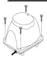
1. Remove cover bolts using a 8mm-box wrench.
