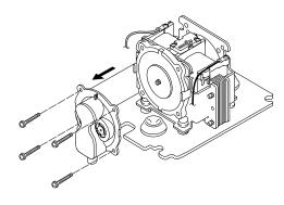
4. Remove 4 screws from a casing using a cross slot screwdriver.
