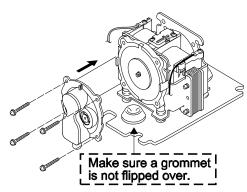
7. Insert a casing air outlet into a rubber grommet and fix a casing assembly with 4 screws.
