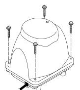
10. Fix cover bolts using a 8mm-box wrench.
