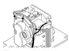
8. Fit a power cable in 3 hooks.
