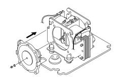
6. Place a new diaphragm using new nut provided.
